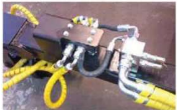
Press button, 6 way valve and double safety valve
