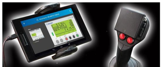
7" tablet as a measuring device display. Radio control button attached to the crane operating handle.
