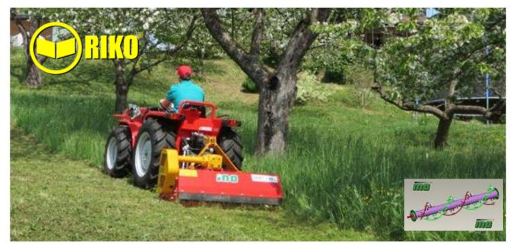
FLAIL MOWER MMT 14 - 30 KW (19-40 HP)
